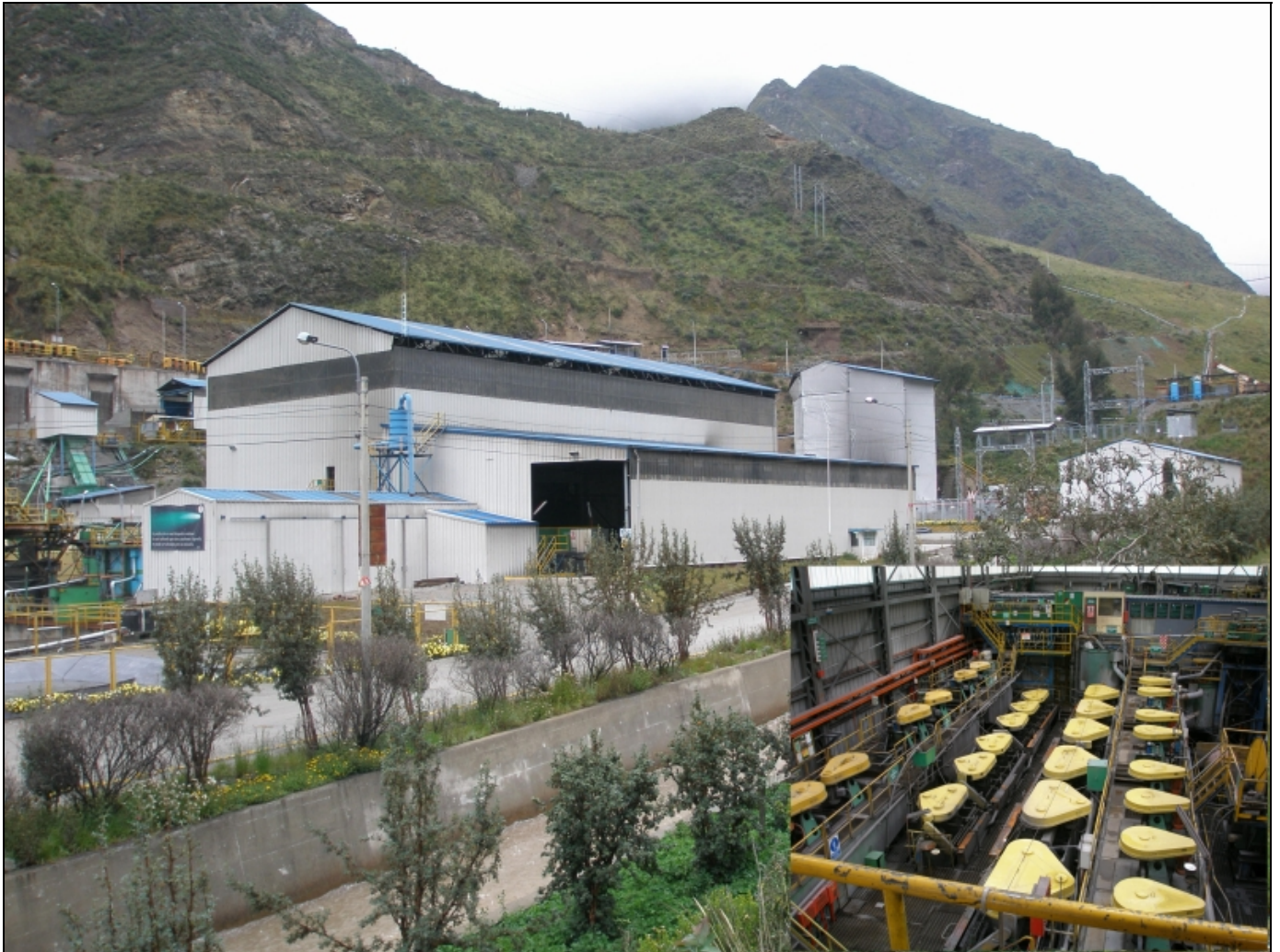
Figure 1. Glencore's mill and processing plant (inset, flotation cells) to be mobilized to Santander mine project.
